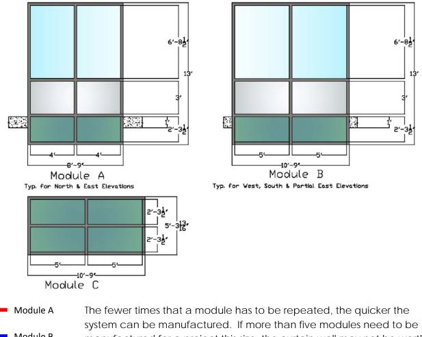
Module A The fewer times that a module has to be repeated, the quicker the system can be manufactured. If more than five modules need to be manufactured for a project this size, the curtain wall may not be worth building as a modular system. Three modules, as seen below, were designed for the library's new façade.
