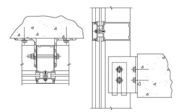
With a stick-built system, the connection penetrates the concrete slab horizontally, which is opposite from a unitized system.
