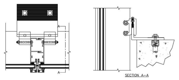
With a unitized system, the connection penetrates the concrete slab vertically, resting on top of the slab.
